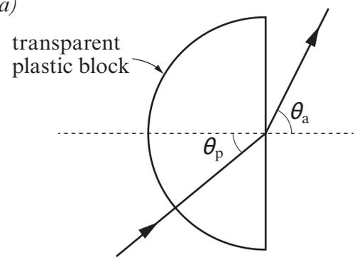
A student traces the path of a narrow beam of light through a transparent plastic block, and measures the angles  $\theta_a$  and  $\theta_p$  (see diagram). She repeats the measurements for various chosen values of  $\theta_p$ , and her results are plotted below.
