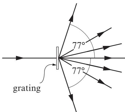
A diffraction grating with  $5.00 \times 10^5$  slits per metre is used to measure the wavelength of the laser light, which is shone normally on to the grating. The emerging beams (see diagram) are found to leave the grating as shown.
